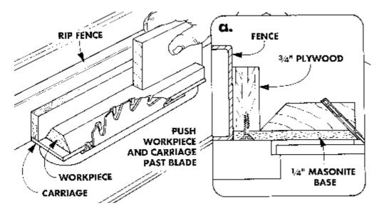
To cut the second bevel, I built a carriage, see drawing. The work piece rests on the carriage and the two are pushed along the rip fence together. This way the edge of the first bevel can't get jammed under the fence. And it's protected from damage.
